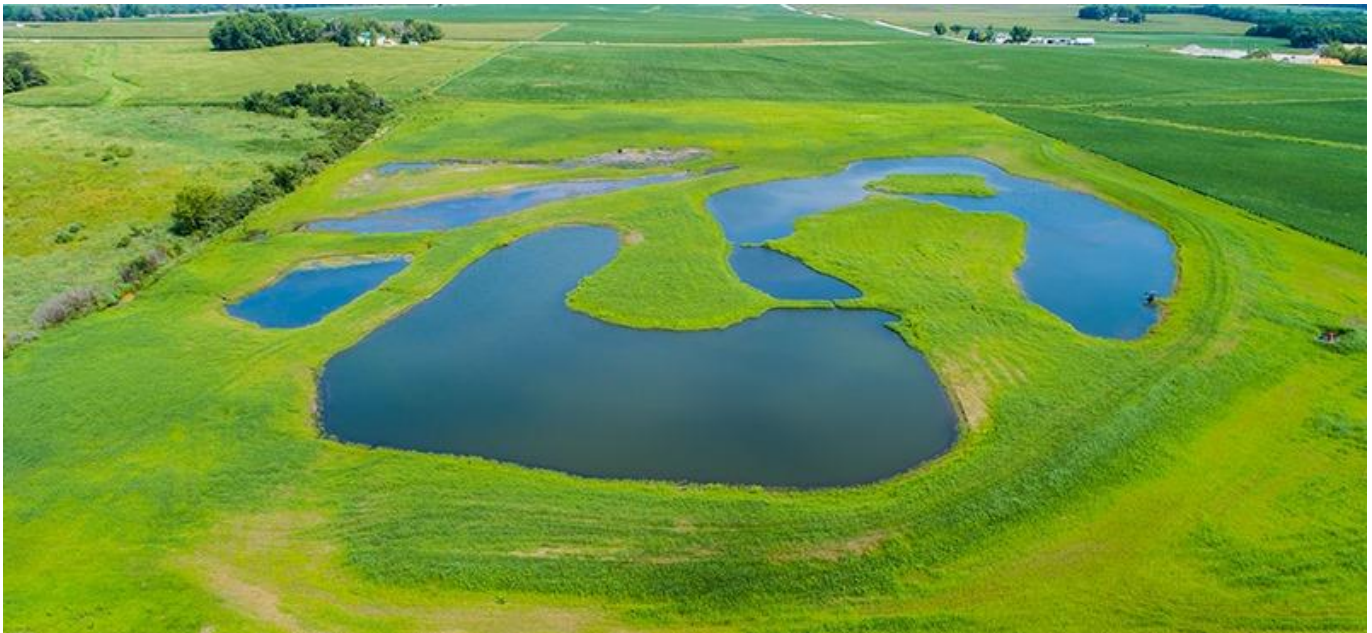
Figure 7. The Albert Wetland project installed in the Middle Cedar River Watershed has a drainage area of 112 acres, a pool of 8.5 acres, and an approximate cost of $148,500.
