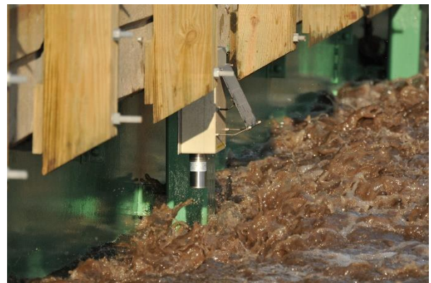
Figure 2. IFC stream-stage sensor in action.
